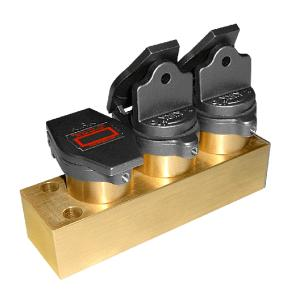
The Type T interlock is an assembly of two or more lock cylinders in a single housing. Type T interlocks are designed to retain one or more keys (called held keys) while the remaining (initiating) key(s) are removed. This allows an exchange of keys in an interlock sequence. All initiating keys must be inserted into the Type T interlock before the held keys can be removed. Once a held key is removed, the initiating keys are trapped in the interlock.
